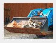
**High Capacity Front Loader** Features 1,276 lbs. of lift
