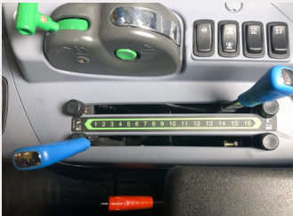
Position and Draft Control Three Point Accommodates a variety of implement needs
