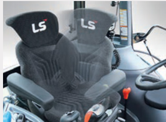
Premium Seat The air suspension seat with 10 degree swivel for added comfort
