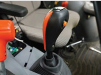
Hand Clutch The hand clutch button added to the gear control lever enables you to change gears easily
