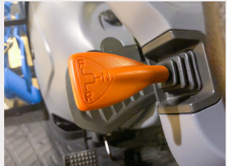
Power Shuttle Transmission Enables fast and efficient directional changes (CPS) model only)
