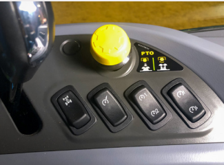
Electric Engaged Independent PTO Readily available to the operator to control PTO implements
