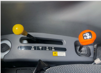
540/750/1000 PTO Provides compatibility to a large number of implementst
