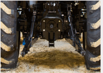
High Capacity Three Point Hitch Heavy-duty frame and lift cylinders enable three-point lift capacity of 2,755 lbs. at hitch end
