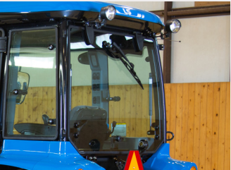
Rear Window Wiper, Cab Model Deluxe feature for better visibility and safety
