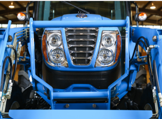
Standard Factory Grille Guard W/ Loader Full length grille guard protects body panels and radiator
