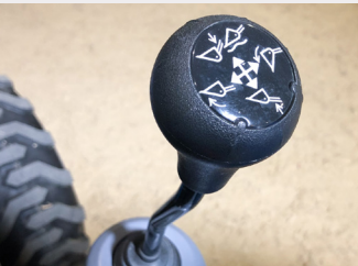
Integrated Joystick Provides comfortable access for loader operations. 3rd function (option)
