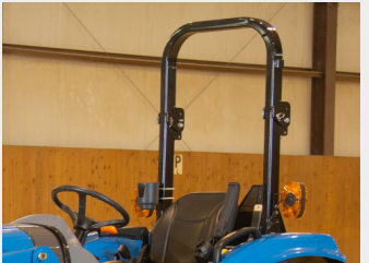
Standard Foldable ROPS Provides clearance options
