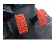
3 Range Hydrostatic Transmission, (2 Pedal) Comfortable And Efficient **Operator Control**
