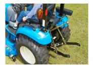
**Durable And Adjustable Three Point** Provides 1,433 lbs. Of Lift Capacity
