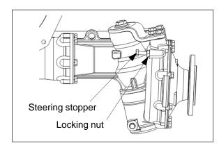
5) Tighten the locking nuts of the each side.
