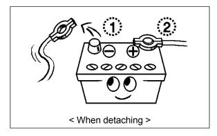
When attaching the battery, the positive (+) terminal must be attached first and the negative (-) terminal must be connected last.
