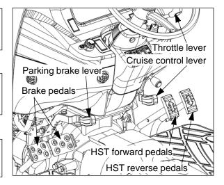
▶ If pressing brake pedals or HST forward pedal down deeper, the cruise control drive shall be stopped.
